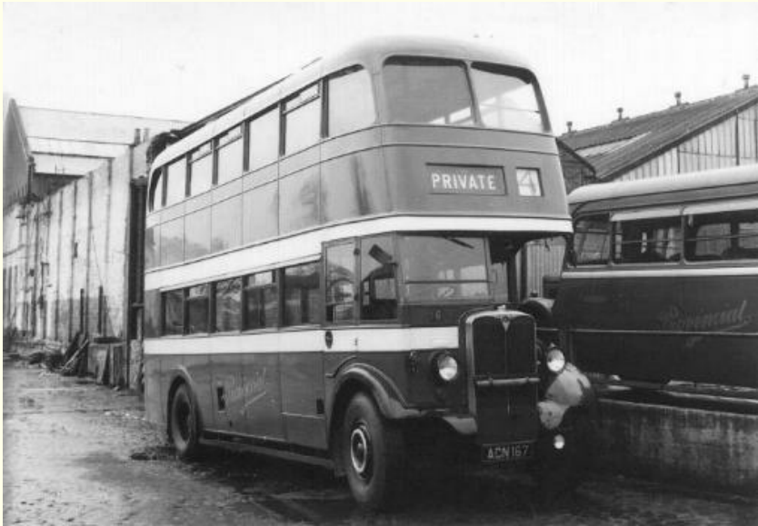
16 (ACN 167) seen here at Hoeford with a temporary route number. 16 was new to Northern General as No.1167 in 1946. It is an AEC Regent II with NCB body.
