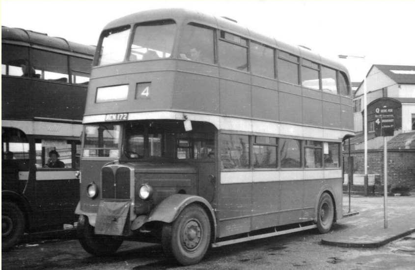
Regent 33 (ACN 172) at the Ferry in January 1958 still in undercoat and without a fleetname. This bus was found to be suffering from rot, so did not last in service very long. The chassis, however, was used as the basis for the AEC-Ruston rebuild 14 (270 MHO).
