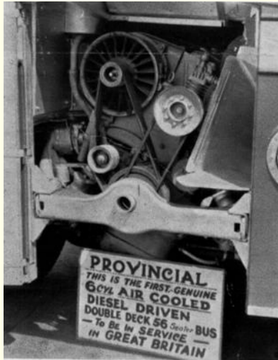
Engine installation - grille panel opened . Photo: The Transport Journal
