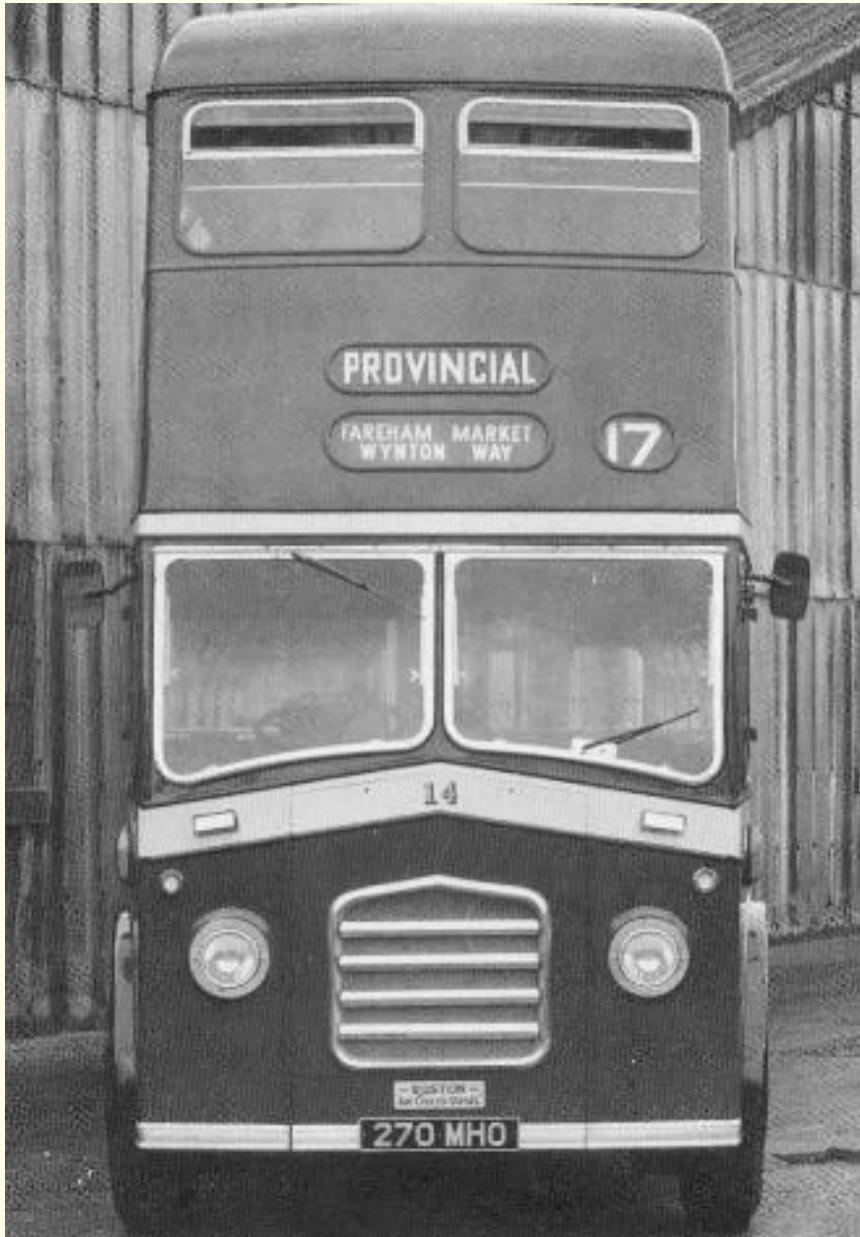
Close up of the front of no.14, showing Ruston badge with phrase "Ruston Air Cooled Diesel". Compare this with the photo on the previous page and you will see two further ventilators have been added. The engine and cab temperature must have been unacceptable.
