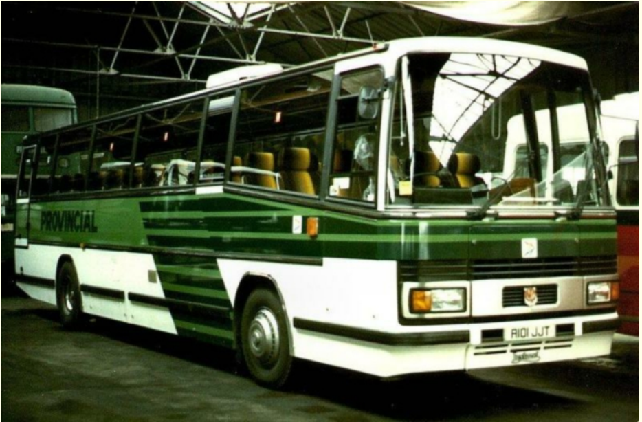
A 1984 Leyland Tiger No. 101 (A101 JJT) A semi-automatic with Plaxton Paramount coachwork.
