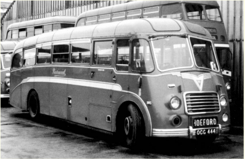
68 (OCG 444) seen at Hoeford. This was one of the coaches rebuilt from AEC Regent Chassis.
