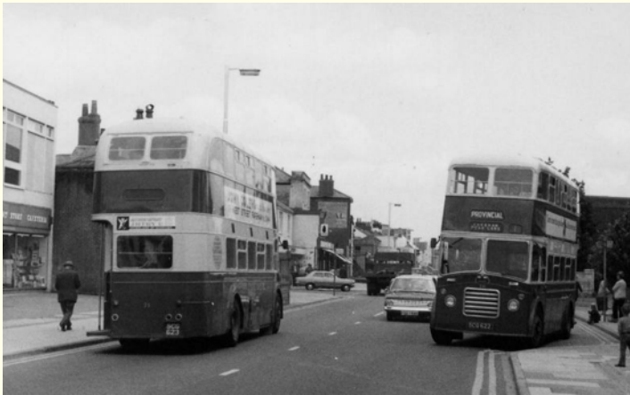
The last two new double deckers delivered to GFOC 70/71 (SCG 622/623) pass each other outside Mc Ilroy's at the location described above. They were Guy Arabs IVs with Reading H30/26R bodies. Photo: Fred York
