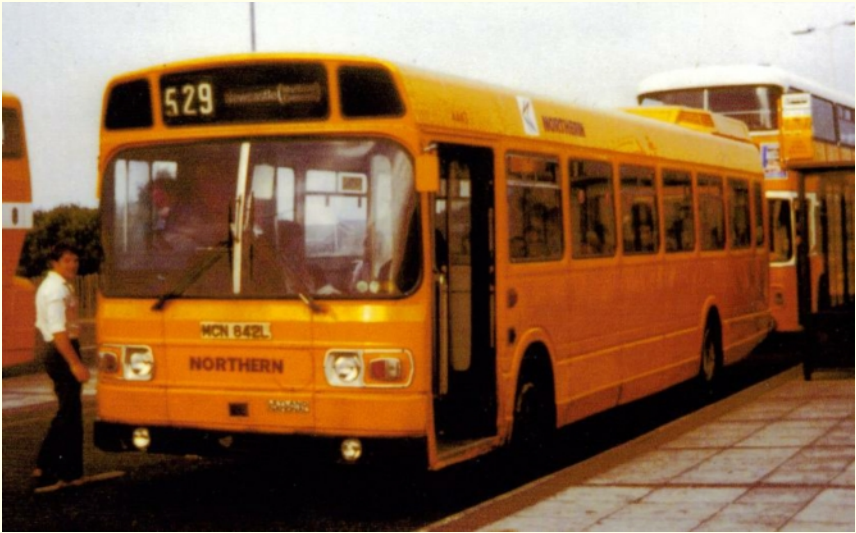
MCN 842L was one of 3 Leyland Nationals to make the long journey from the North East to Hoeford in 1983. When new it was a dual door vehicle, but was rebuilt to single door in late 1979.
