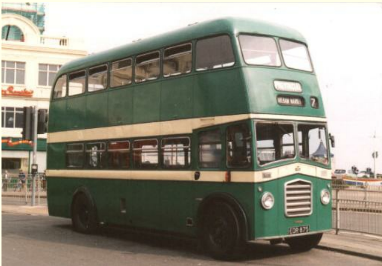
The last Arab to be re-bodied without a Deutz engine was 17 (EOR 875), this was in 1958. This vehicle is now preserved. The body differed from No 60 by having a peak to the front grille and hopper type opening windows.
