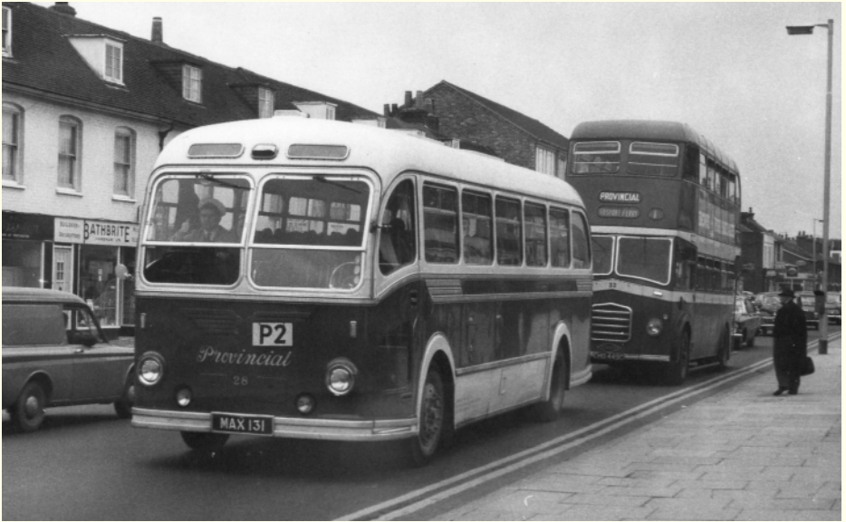
No 28 (MAX 131) an ECW coach bodied Bristol LS6G seen in West Street Fareham, on Foster Wheeler contract duties. Photo: Fred York
