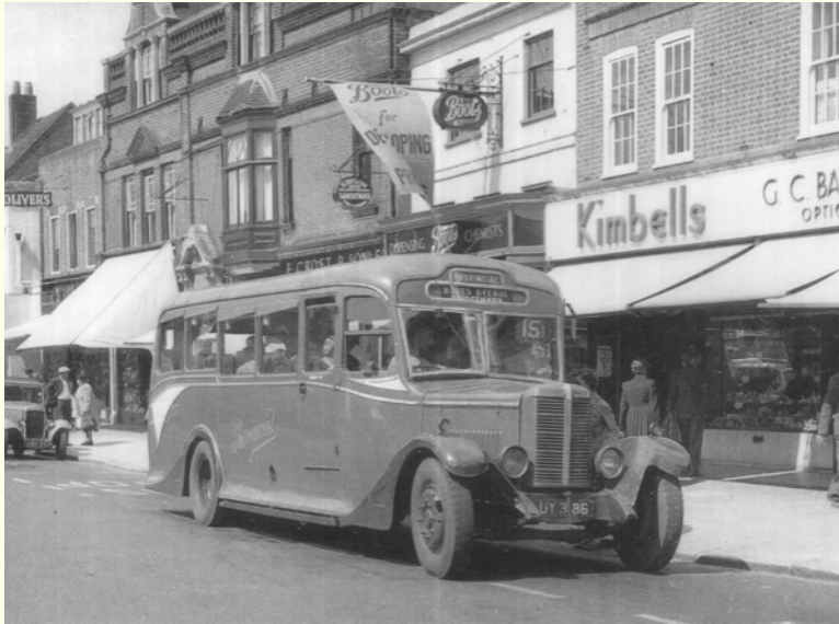
A rather strange vehicle acquired from Premier of Gosport in 1950. No 1 (UY 3186), a 1928 Maudslay ML4 with a Bedford OB radiator and Grose bodywork. this stayed with Provincial for 4 years.
