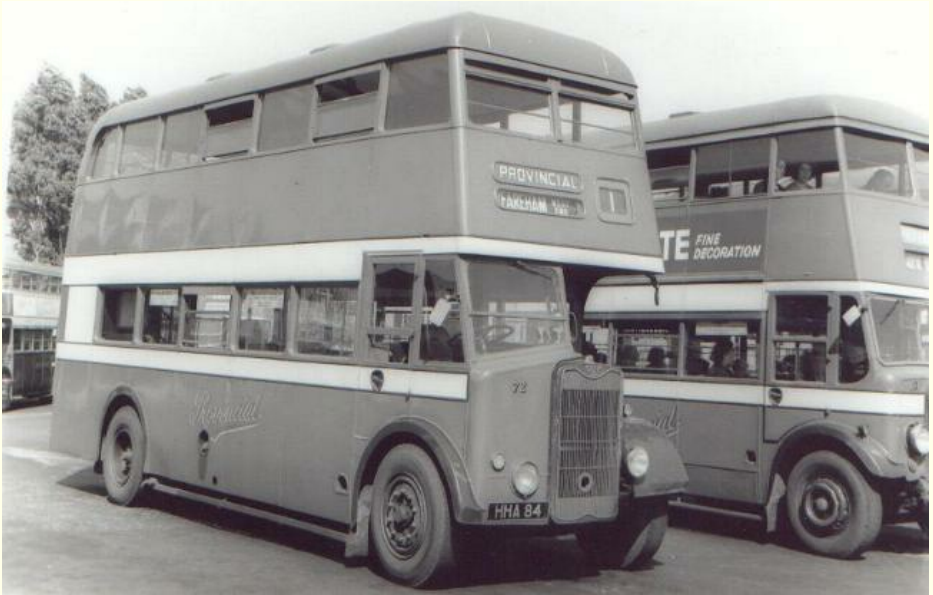
No 72 (HHA 84) is seen at Gosport Ferry. The built up front nearside wing fitted by BMMO by Hooten has been replaced, detracting from the balanced lines of the body.
