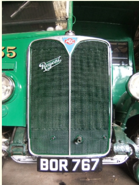
From 1937/38 most AECs were built with a 'long' radiator and covered dumb irons to improve appearance. David says :- "I had always wanted 35 to feature the original 'short' radiator'. Two friends, Ian and Jon created the correct radiator in 2023 and Jon also produced the hand painted registration plate" Photo: David Whitaker
