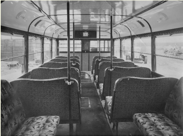
Above: The interior of No. 36 showing the clock and inner panels with a floral pattern. These were in rexine on very thin plywood. They included small metal gauze buttons to allow air to circulate behind the panels. In practice, most of these were severely damaged by small boys who could not resist putting their fingers through them. In later days, Orme White removed all these inner panels. Photo: David Whitaker
