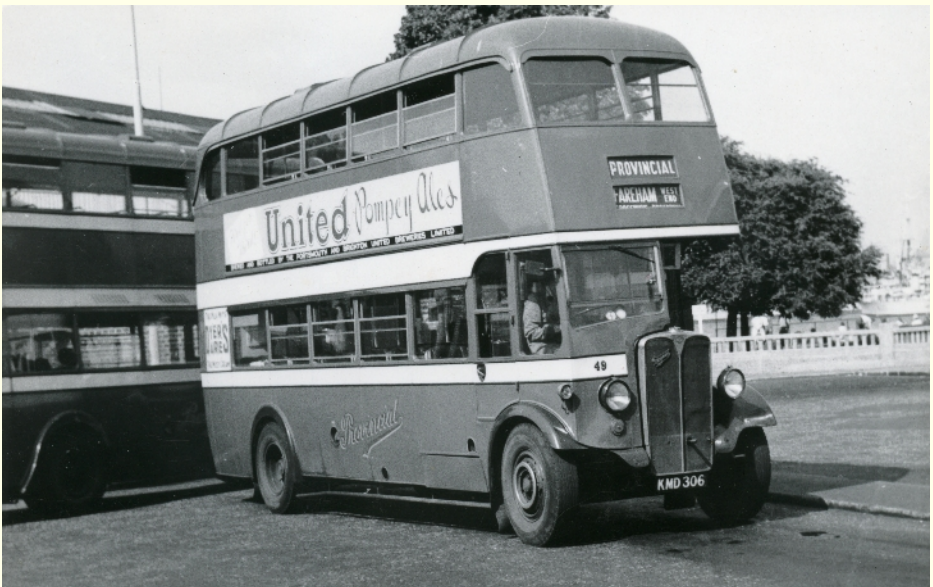
No. 49 (KMD 306) at Gosport Ferry in a position not far from the new bus station. The Park Royal body can be compared to the Weymann body on No. 48.
