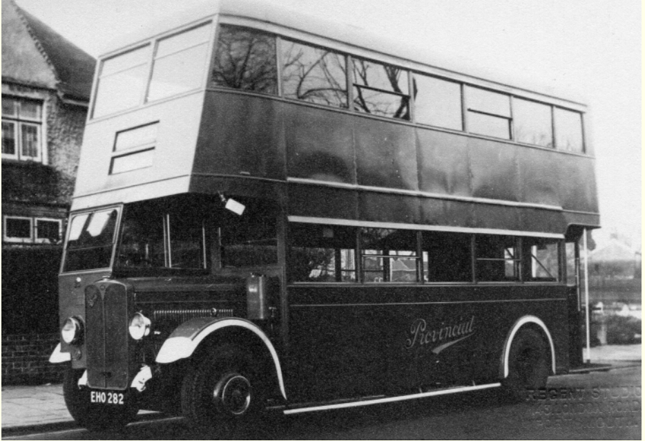
No.15 (EHO 282) seen here in Wartime livery with its original body This was the first double deck body built by Reading, and was modified by them in 1951. It was later transferred to AEC Regent No.12 (FHO 604) in 1960. Photo: David Whitaker Collection
