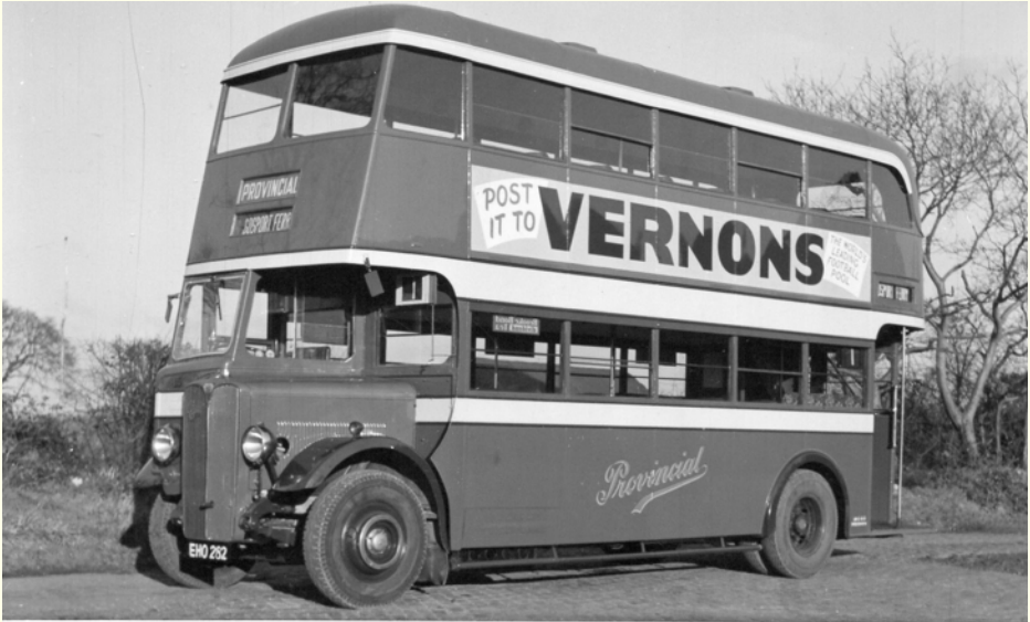
No.15 (EHO 282) is seen here with its 1951 modified body looking a lot more like later Reading products. Photo: David Whitaker Collection
