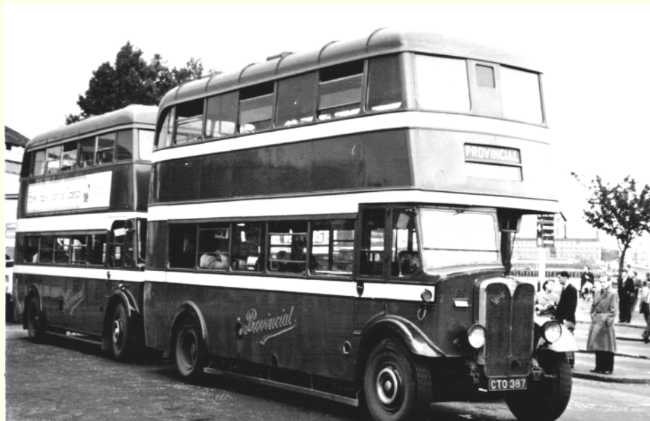
Above: No. 63 (CTO 387) at Gosport Ferry. A unique feature of this bus in the Provincial fleet, was Nottingham's fitting of a route number box between the upper front windows, although this was not used by Provincial. Photo: Stephen Didymus Collection
