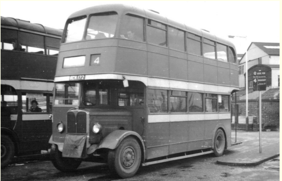
Regent 33 (ACN 172) at the Ferry in January 1958 still in undercoat and without a fleetname. This bus was found to be suffering from rot, so did not last in service very long. The chassis, however, was used as the basis for the AEC-Ruston rebuild 14 (270 MHO). Photo: Alan Lambert
