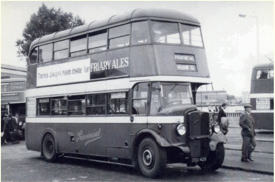
No. 51 (DOU 428) at Gosport Ferry. A couple of points of interest are the radiator blind which was used to reduce cooling in the Winter months. Also, the route number indicator is carried under the nearside front canopy, a temporary measure until the bus went through a body overhaul when a route number aperture was added next to the destination blind. Photo: Provincial Society Collection
